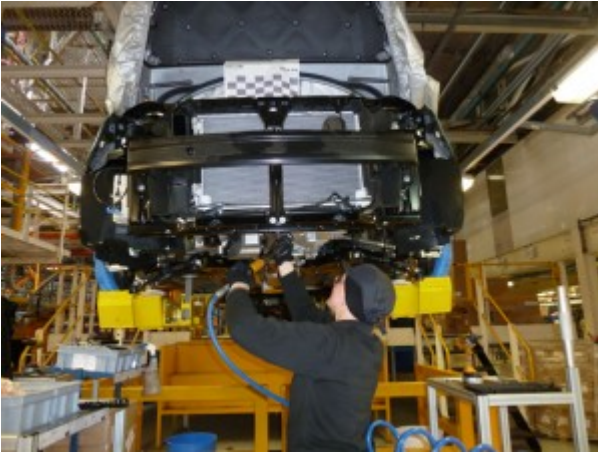
The engine/transmission/steering/front sub-frame assembly is raised into position from below, and bolted in (Lisa Ponter working here; please see text).
