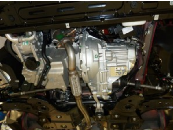
This is the engine/transmission assembly viewed from below, shown now with the exhaust system attached.
