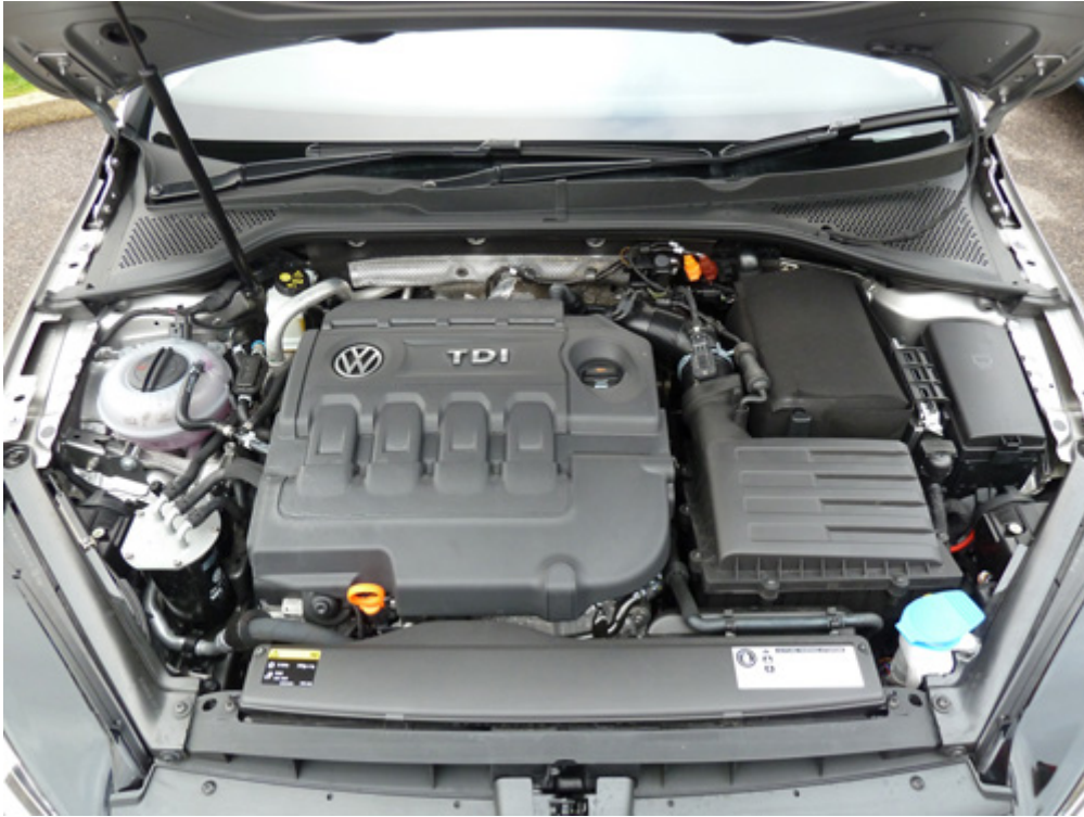
The 1.6 litre diesel engine fills most of the available underbonnet space. It's technically advanced, and returns excellent fuel consumption.
