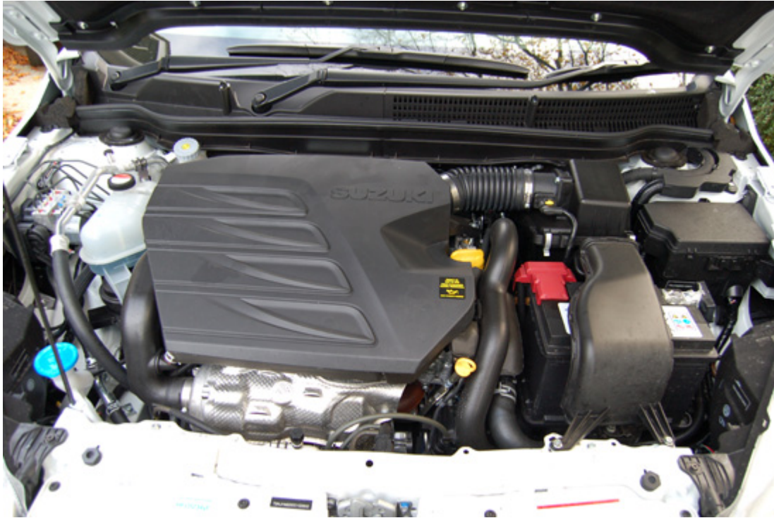
Beneath the plastic cover sits a strong-performing, refined and economical 1.6 litre turbo diesel engine, featuring a Variable Geometry Turbocharger.
