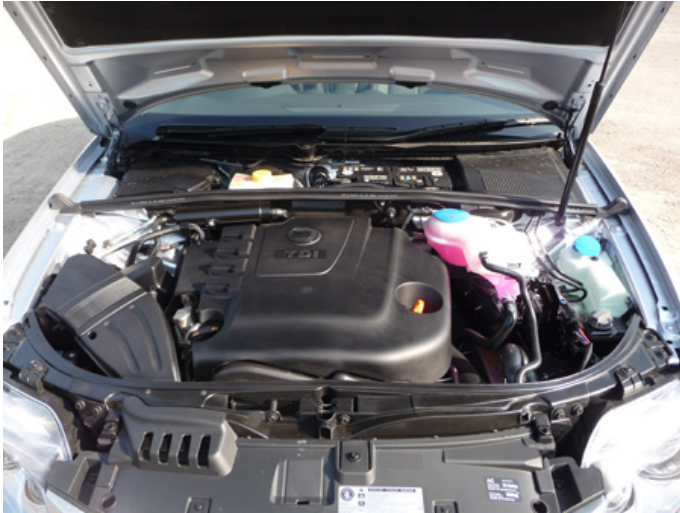
The two litre four cylinder turbo diesel engine develops 143PS; it's a refined and willing unit.
