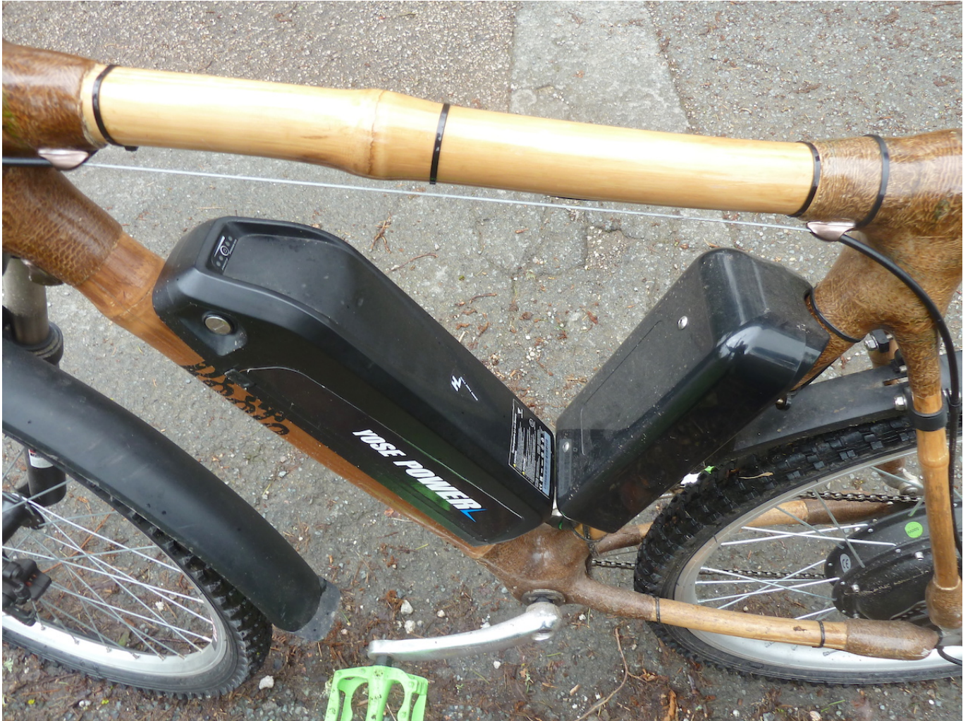
Battery pack mounted within the frame, on the electric version.
