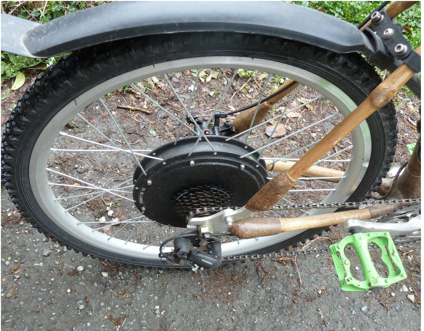
Rear hub-mounted motor on the electric model.
