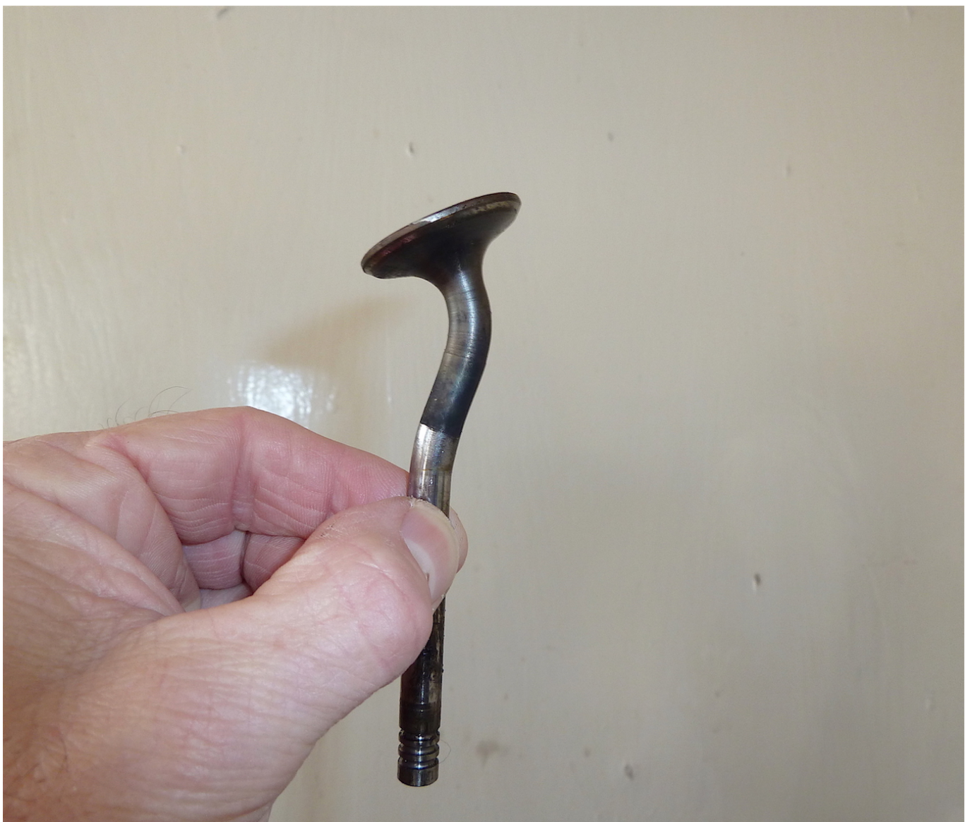
A very bent valve; the result of cam belt breakage in a 2008 Ford Mondeo...
