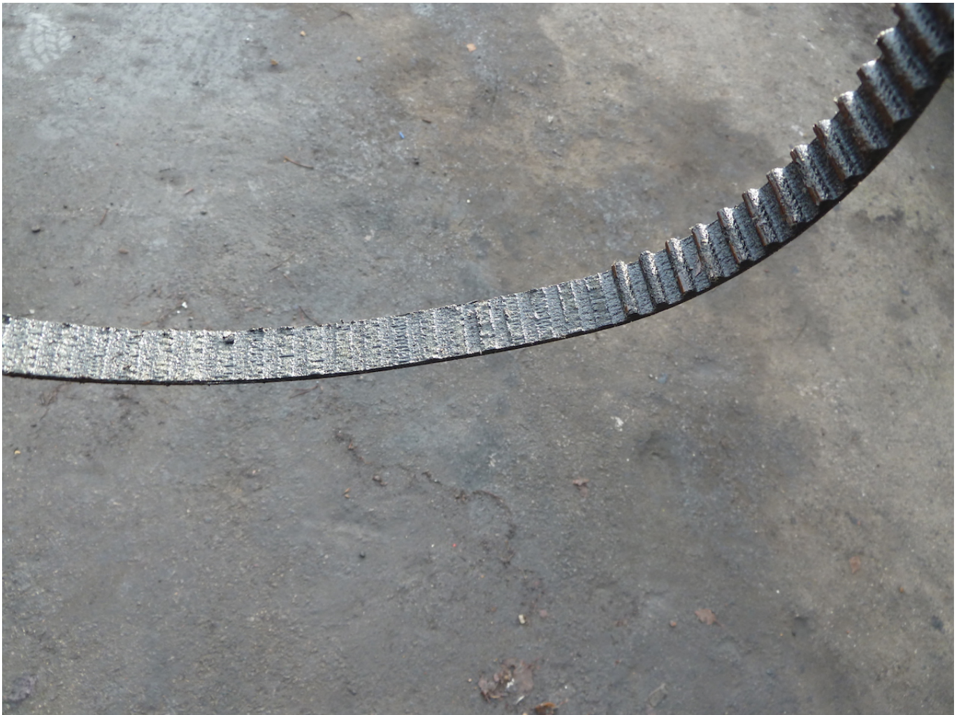
Drive teeth stripped from a Mondeo cam belt that had been overdue for a change.
