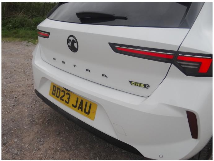
Motive power for the GSe comes from a 186 PS four-cylinder turbocharged 1.6 litre petrol engine accompanied by an  $81.2~\mathrm{kW}$  (110 PS) electric motor; these work together for a combined total power output of 225 PS and maximum torque of 360 Nm (266 lb.ft) and apply this to the front wheels via an eight speed automatic transmission.
