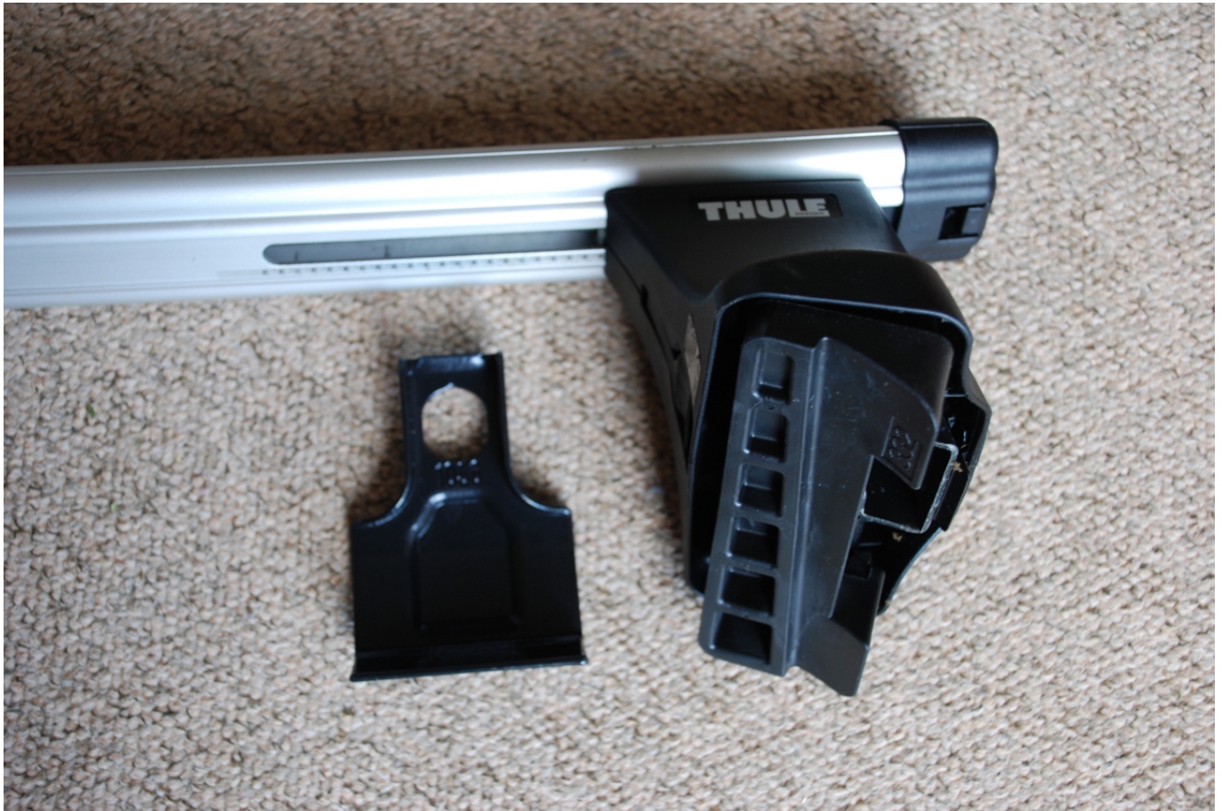
Above: The foot with the 'claw' ready to be fitted...
