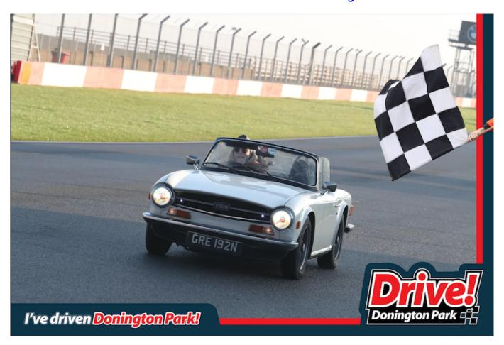
The Triumph TR6, the sports car in our convoy. A 2.5 litre fuel injected in-line six engine, providing 150bhp and 143lb ft of torque to the rear wheels via a 4-speed manual gearbox with overdrive. Taking the chequered flag, far from the top speed of 119 mph, Giles looks like a naughty schoolboy following his wee mishap a few corners prior.
