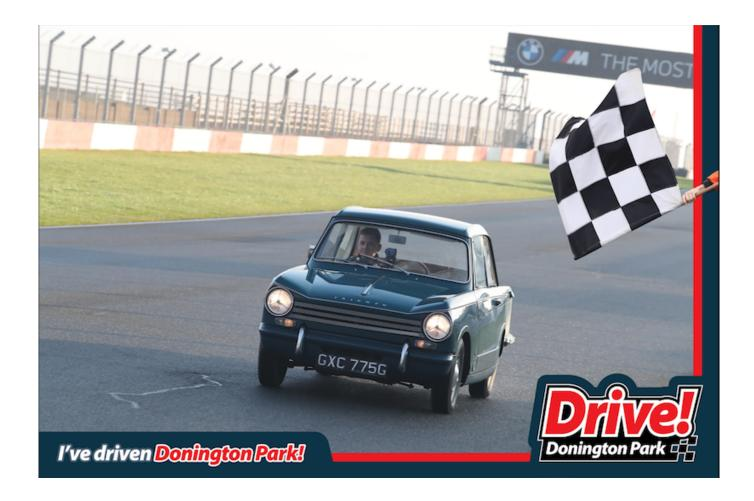
My 1969 Triumph Herald 13/60, a small 60s family car. The little 1.3 litre in-line four only squeezes out 63 bhp and 73 lb ft of torque, but it is relatively light, and in my three years of ownership I have carried out some subtle performance upgrades, such as uprated spark plugs, coil, HT leads and electronic ignition. With that considered, the Herald is more at home on a B-road, and I only hit 60 mph, short of my top speed of 85 mph, but was still ample fun on track.
