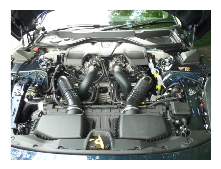
The twin-turbo motor takes advantage of patented pre-chamber combustion technology and features twinned spark plugs, these aspects developed to help win races but applied by the makers to provide 'extraordinary performance' on the road too.
