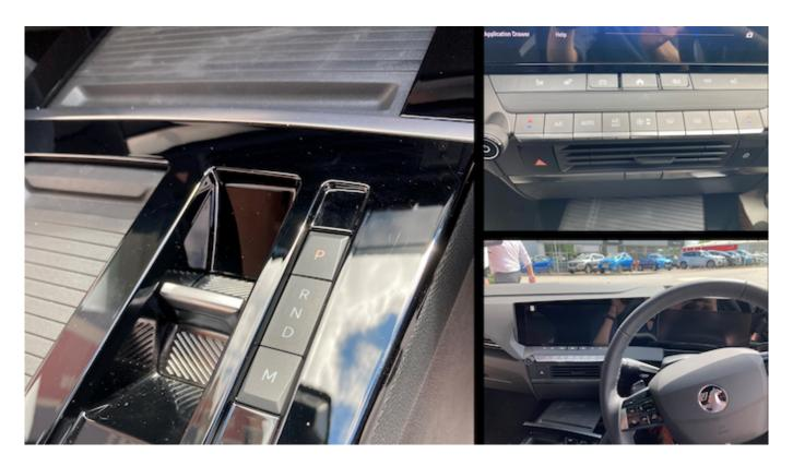
The Astra comes with either a 5-speed manual, or an 8-speed automatic gearbox. Note – the manual is only available with the petrol variants, whereas the diesel and hybrid variants utilise the automatic box. In terms of practicality, the manual takes up a storage area in the centre console underneath the HVAC controls, and the automatic setup reduces the centre
