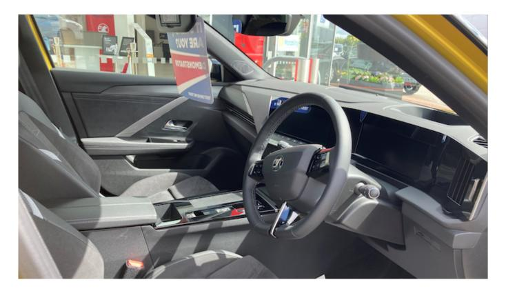
As standard, all Astra models feature a wraparound multimedia system that includes a 10-inch colour touchscreen which is angled towards the driver, and a 10-inch digital instrument cluster, along with wireless Apple CarPlay and Android Auto. The driver's display has been
