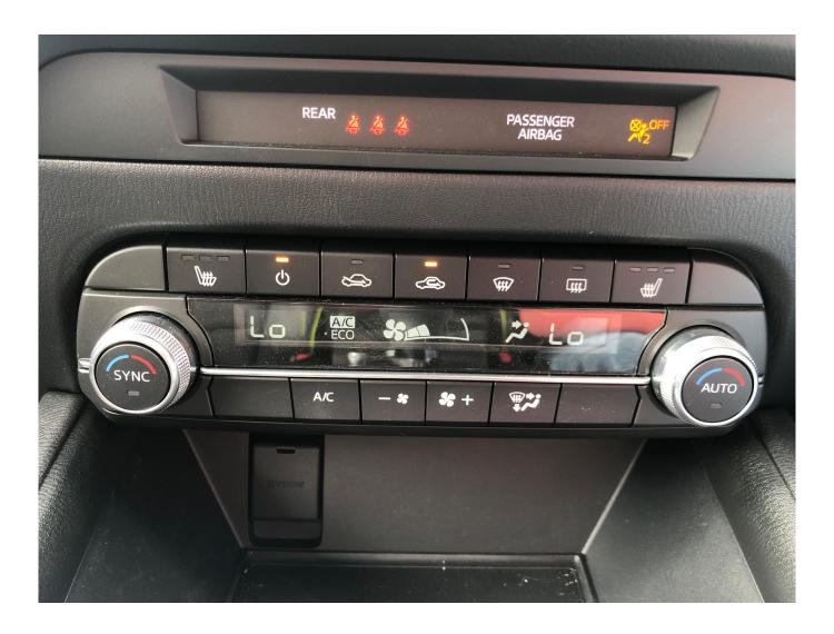
Heating and ventilation was covered by switches on the central console and the system worked well with good markings and effective output, direction and temperature controls.
