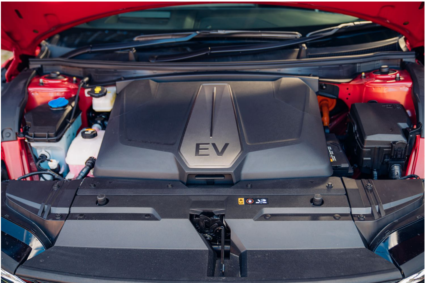
Under the EV6's bonnet is the electric motor (with a storage box on top!).
