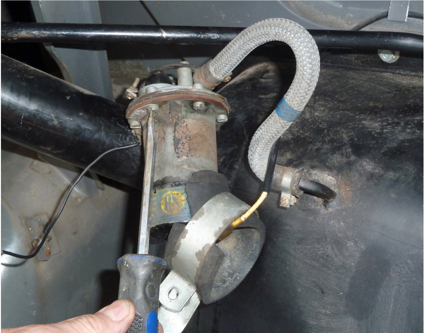
Older vehicle petrol pumps, hoses, seals, floats, etc. - all at risk when ethanol is in the fuel mix.
