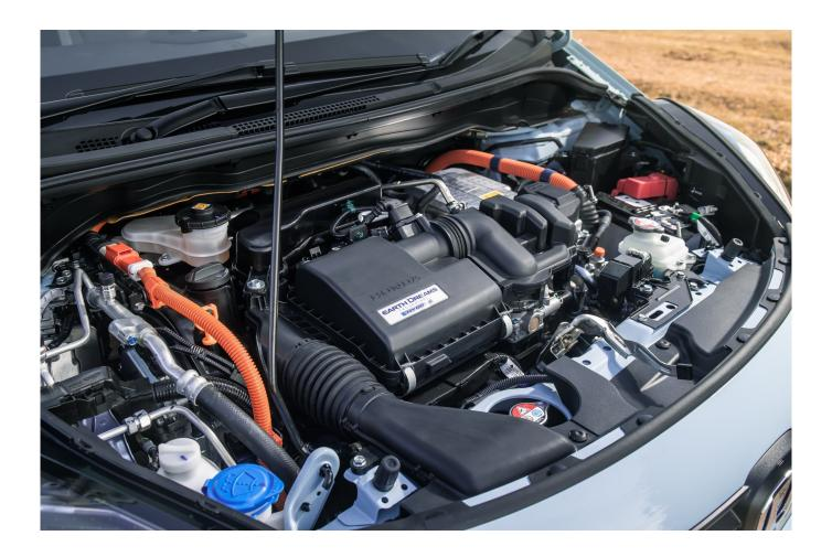
In most urban driving situations best efficiency is achieved with transitions between EV Drive and Hybrid Drive. For driving at motorway speeds, Engine Drive is used, supplemented by an on-demand peak power 'boost' from the electric propulsion motor for faster acceleration.
