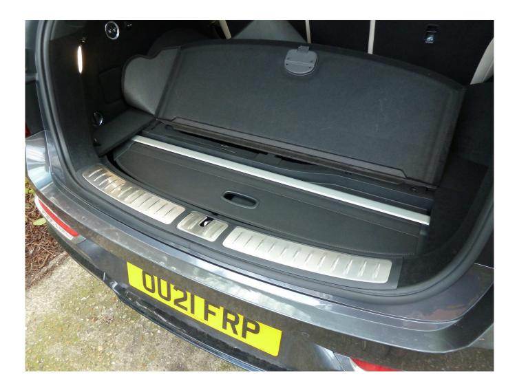
The rear seat backs, divided 2/3:1/3, can be folded forwards by direct activation of the release mechanism at the seats themselves, or by means of a handy button built into the left-hand side wall of the boot. It is worth noting that when restored to their 'upright' positions, the angle of the seat backrests can be set according to choice (they are multi-adjustable).
