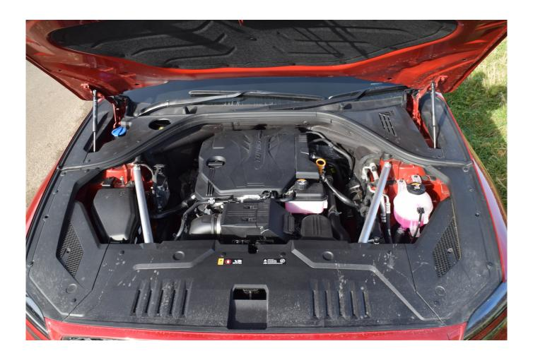
Notable technical aspects include a dual injection fuel delivery system (the dual system enables ultra-precise metering of fuel according to varying driving conditions), and innovative engine cooling arrangements. The 'variable separation' cooling system is said to enhance knocking performance and reduce friction by controlling the flow and temperature of the coolant.
