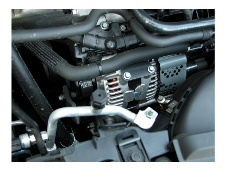
The BISG also acts as a motor integrating with the engine and using the stored energy to provide torque assistance during normal driving and acceleration as well as running the vehicle's electrical ancillaries. Torque output is 240 Nm (177 lb.ft) for the 155 hp Hybrid unit.
