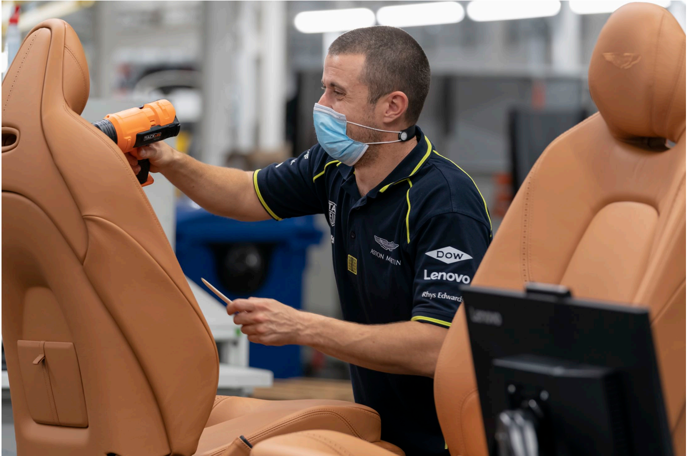
Seats being assembled for the DBX.
