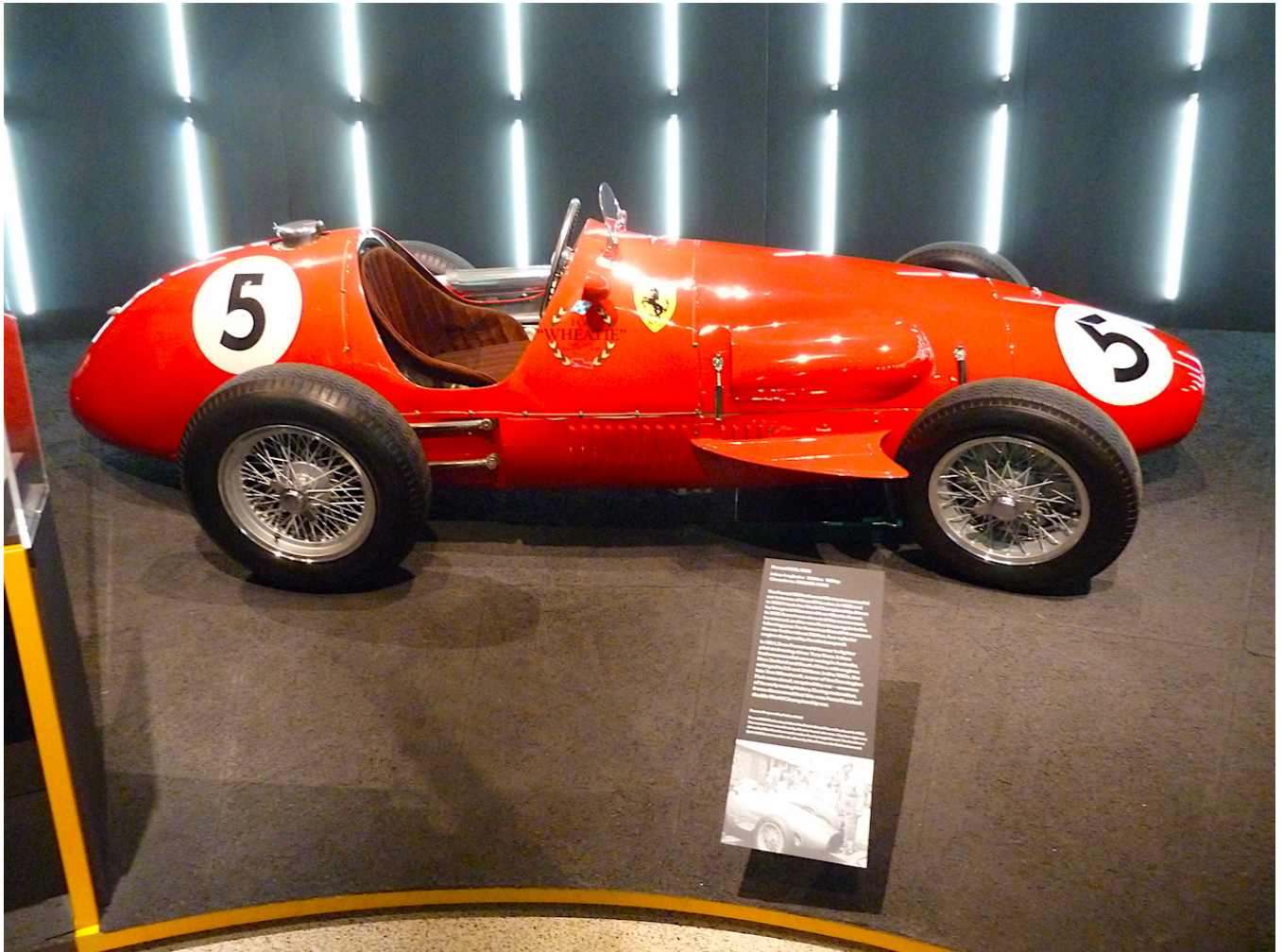
1952 Ferrari 500 (in-line four cylinder engine, 2.0 litres, developing 165 hp). This car won the World Championship in 1952 and 1953, driven by Alberto Ascari.
