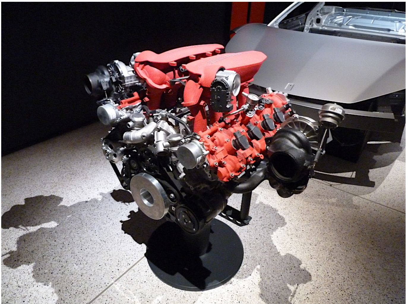
The 3.9 litre V8 motor of the 488 GTB, developing 661 hp.
