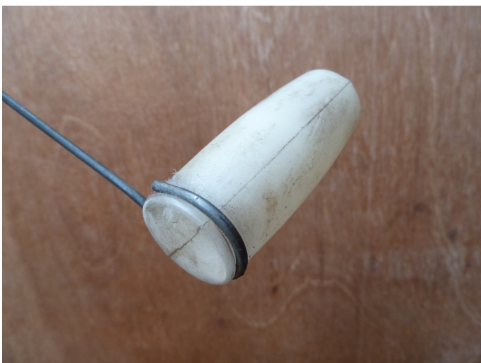
In the future, petrol tank gauge floats will need to be of ethanol-proof materials... (Photo by Kim Henson).
