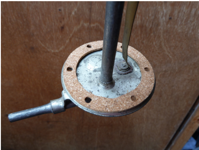
Cork gaskets are among components that suffer with exposure to ethanol... (Photo by Kim Henson).
