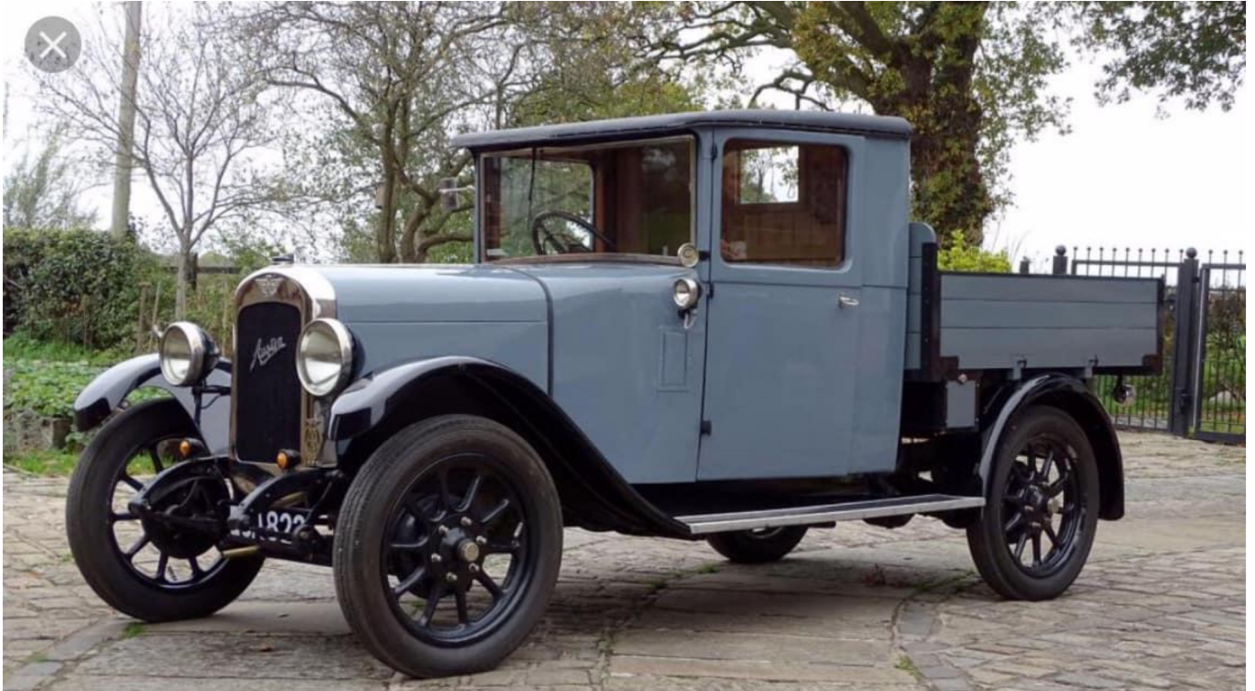
Above: Twelve-Four Longbridge-built works truck. One of several built for internal use from surplus early car parts. Photograph by David Gordon.
