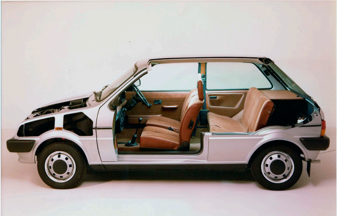
Austin Mini Metro 1.3 HLS 1980. A sectioned car demonstrating packaging and interior space. It was silver with paprika trim.
