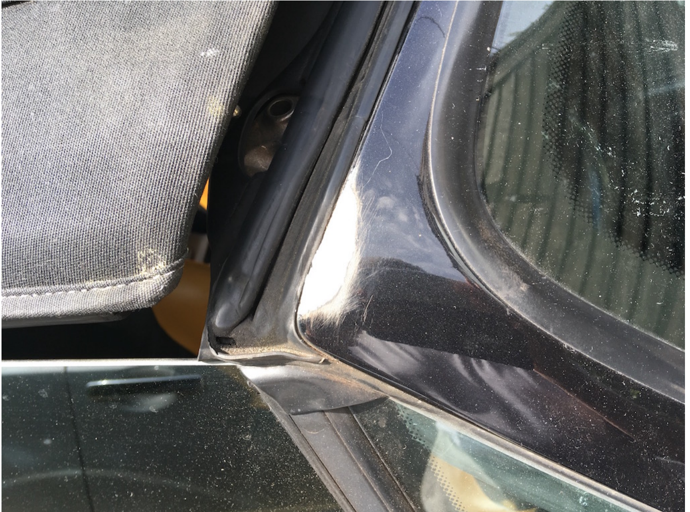
Half a dozen blotchy paint zits treated to DIY undercoat , then touch up paint with variable success!
