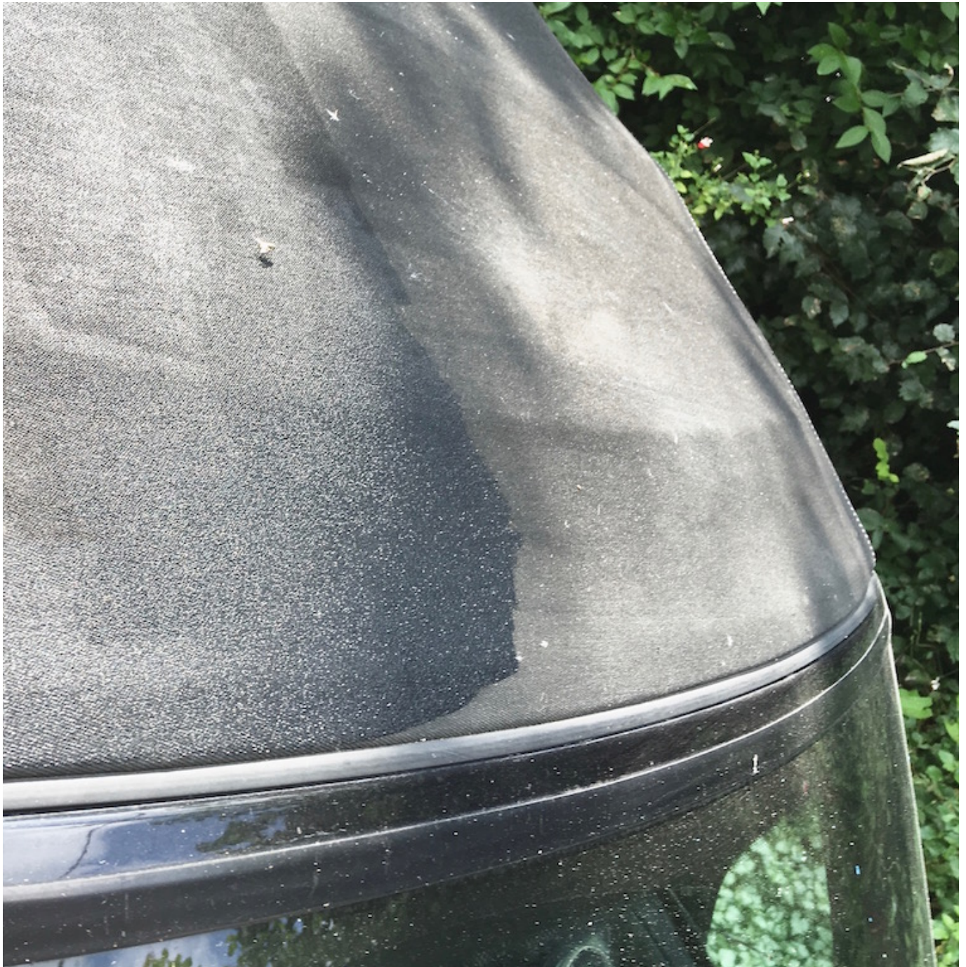
Hood responded magnificently to Renvo treatment in three stages; in progress here.
