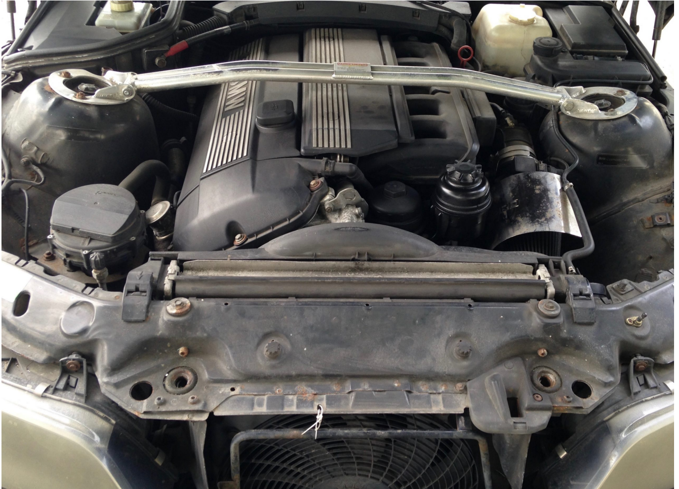
Strut brace delivered taut drive, but needed much polishing!
