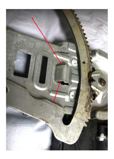
Highlighted by the red arrows are the mechanical stops that are built in to the base of the regulator. These prevent any strain being put on the glass when the window is closed, or on the frame when open. They are set to suit the window size of the Corsa. Needless to say, the A30 windows are smaller!
