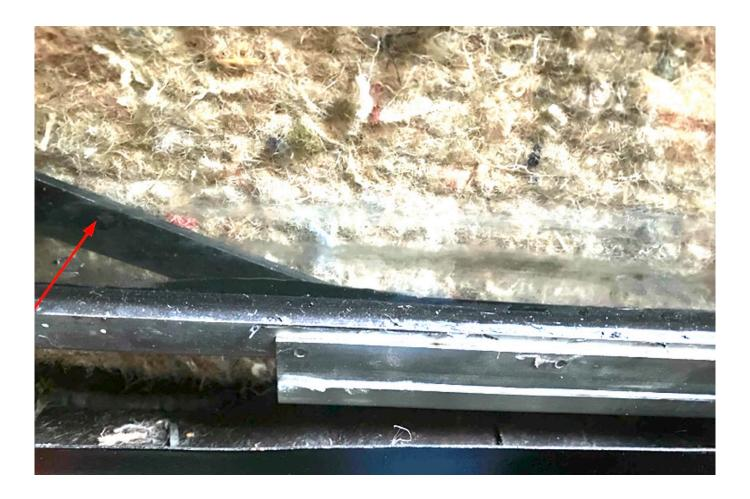
The slider channel is facing away from us in this picture, facing towards the door skin rather than the car interior. This is because the ball joint is pushed into the plastic slider from the rear.
