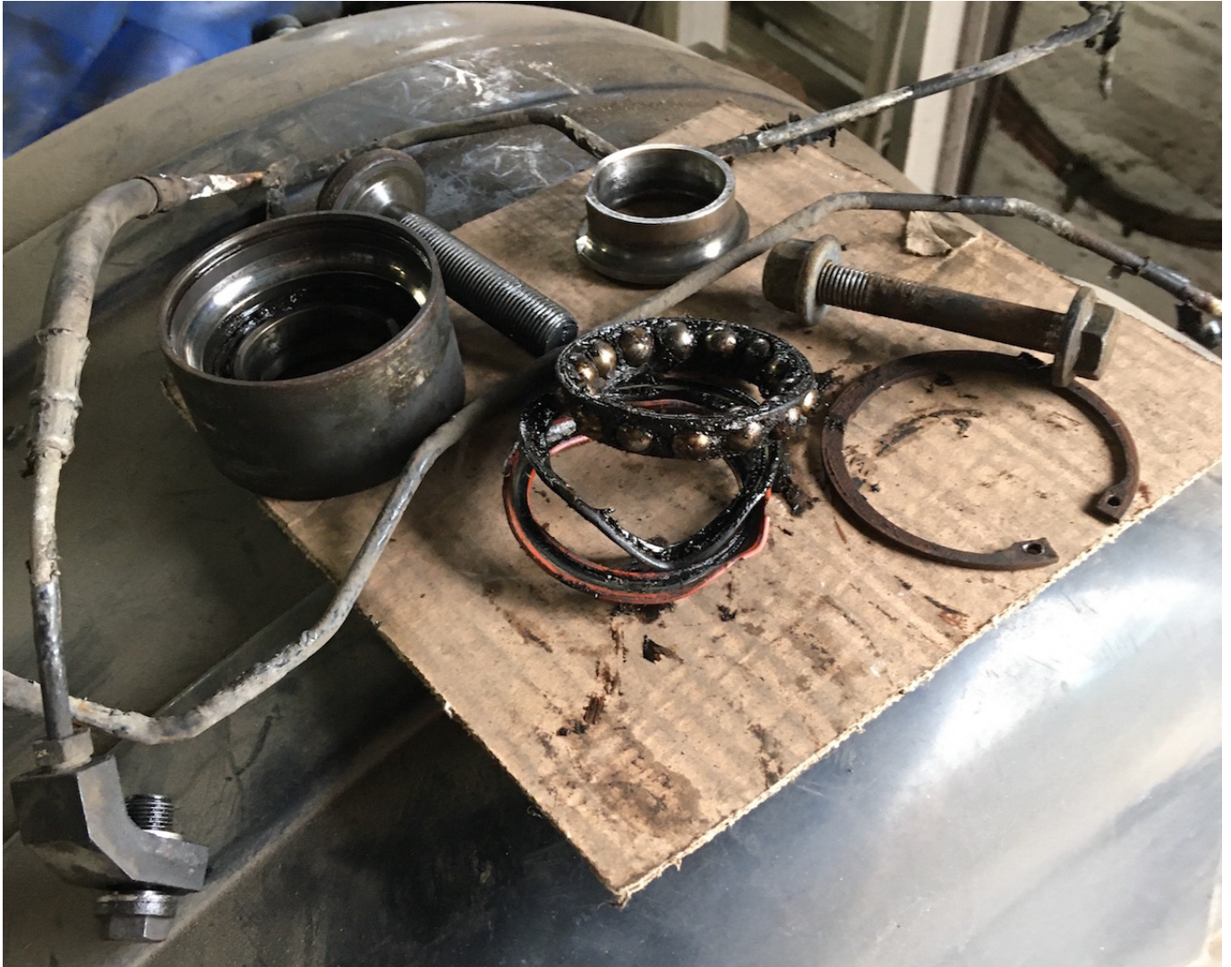
Front wheel bearing race and rear brake lines were necessary and effective maintenance items.
