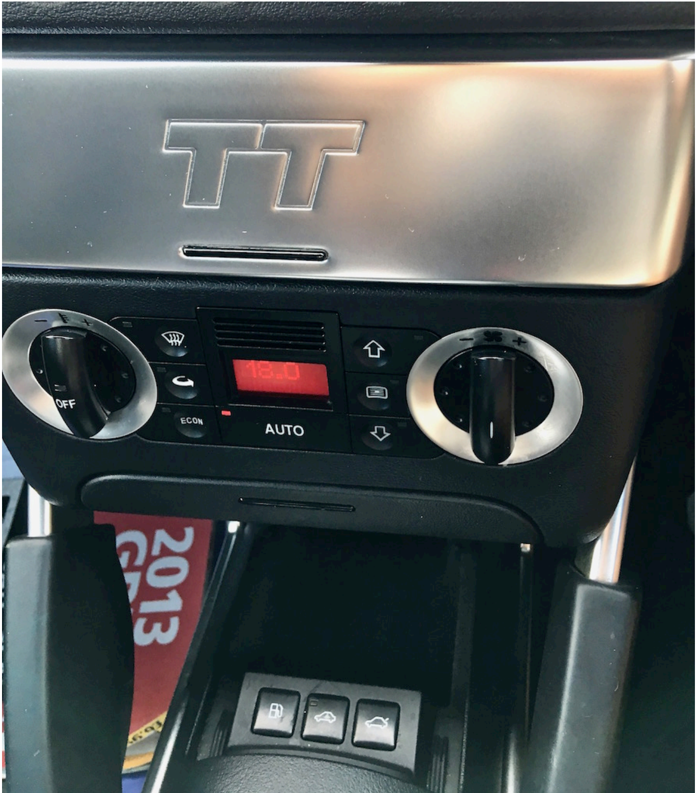
Bose Concert radio concealed beneath TT silver flap, fuel and rear boot releases under
