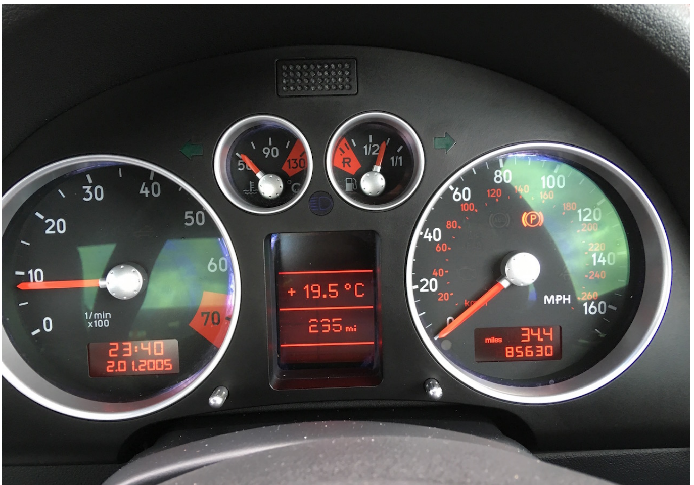
Dials soon after pick up, losing pixels in the centre readout...
