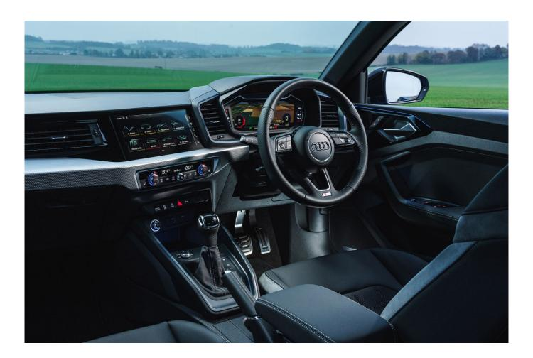
The digital driving instruments were selectable for prominence depending on driving mode and very clear whichever was on screen at any time. They are not the full colour variable type which some other cars use, but they were clear and easy to read as well as being nicely marked.
